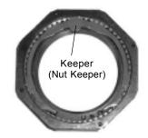
Pro-Torque® Axle Nuts Many Features to Consider: -Longer tread life by controlling axial motion. -Extended seal and bearing service. -Improves ABS by controlling the axial motion.
